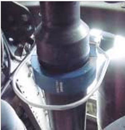
1: Torque measurement on a truck cardan shaft
