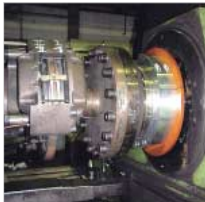
4: Temperature measurement on a brake test stand
