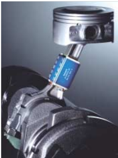
6: Piston temperature measurement
