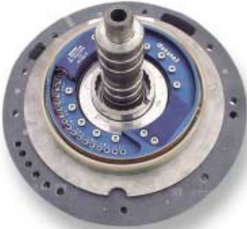
2: Temperature measurement in an automatic transmission
