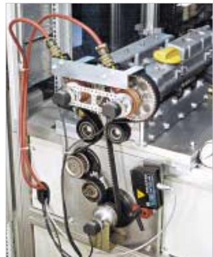
5: Torque measurement on a camshaft test stand
