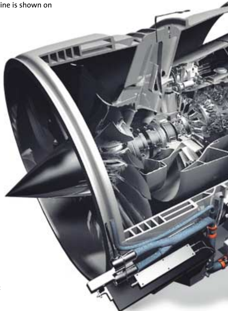
Photo 1: Telemetry installation for LP compressor test on EJ200 engine
