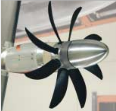
Photo 4: Propeller model with strain gage balance and telemetric data transmission
