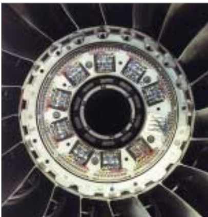
Photo 1: Telemetry installation for LP compressor test on EJ200 engine
