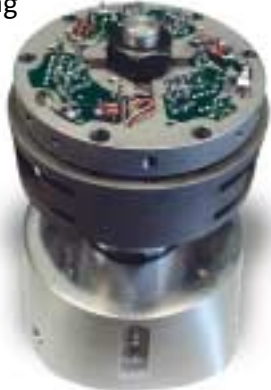
Photo 5: Strain gage balance with integrated transmitter modules
