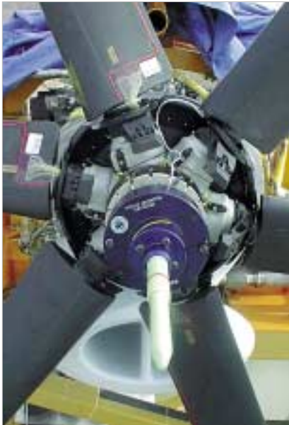
Photo 3: Telemetry transmitter unit mounted on propeller hub
